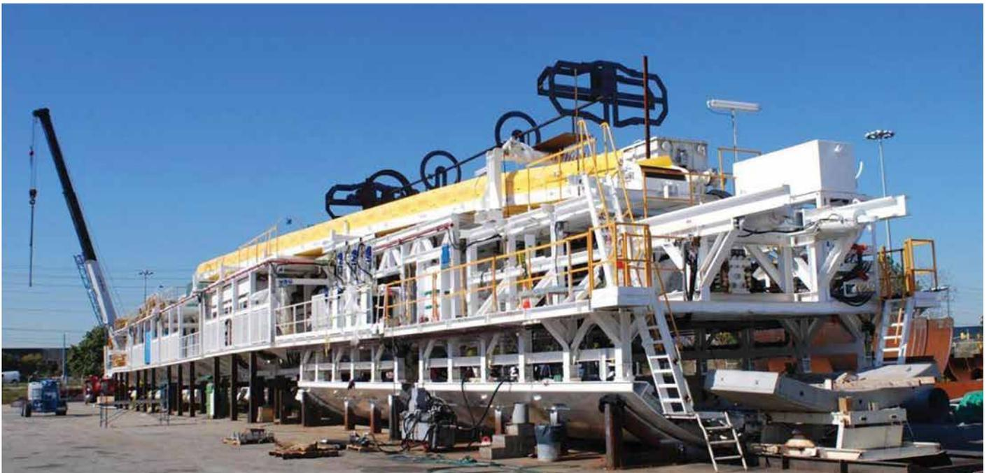
The tunnel boring machine's trailing gear uses a conveyor belt system to remove tunnel spoils and assists in the installation of concrete tunnel liner rings.
