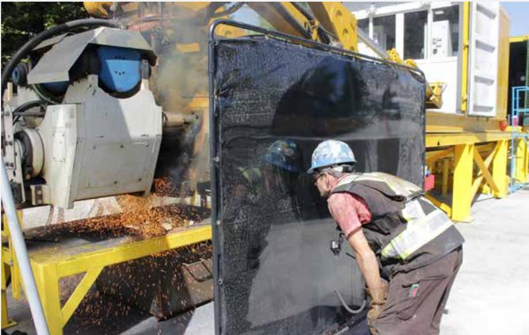
An operator views rails being welded through screen to protect eyesight. Individual rails are welded to make 400 metre sections of track.
