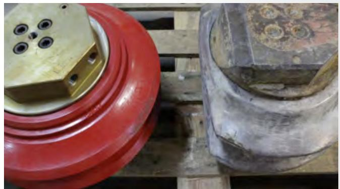
New cutter tool on the left. Worn-out cutter tool on the right.
